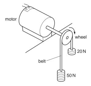
When the wheel is making 20 revolutions per second, what is the output power of the motor?
